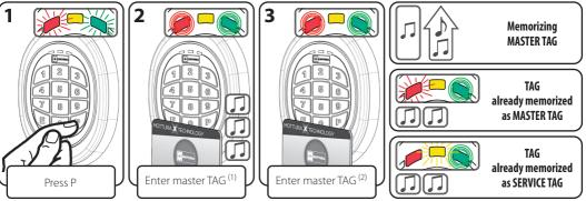
(1) If the lock is new or has been reset, you can enter the programming mode using any free Mottura TAG! (2) which will become a MASTER TAG.
