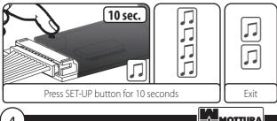
ATTENTION : this operation deletes all tags, pin codes (keypad escutcheon) or authentication (fingerprint escutcheon - note: it does not erase the fingerprints stored in it), and enables the service tags.
